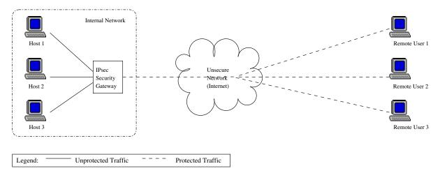
Figure 2: Remote User Access Using IPsec.
