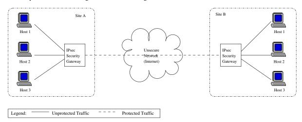
Figure 1: Typical Current Usage of IPsec.
